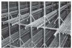
The effectiveness of the fill as a heat transfer medium varies with the size and shape of the splash bars, as well as their vertical and horizontal spacing density. The indicated minimum splash bar spacing is by no means abnormal, and it establishes a datum that assures the fill to be truly non-clogging, and cleanable.
